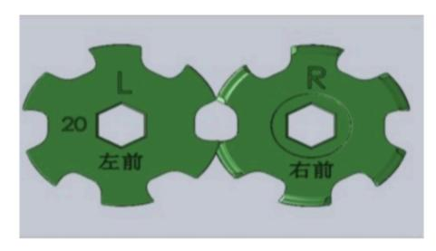
2. When the forming wheel rotates to the position shown in the figure above (the two wheels are easy to disassemble and assemble at this time, and the force on each other is small), turn off the power.
