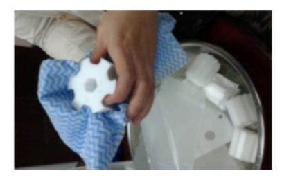
2. When rice is stuck inside the machine, you need to clean and oil it again before operating it.
