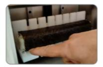
Press the cutting and rolling switch with the index fingers of both hands at the same time.
